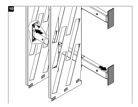
10. Now slide the wall supports of the lower cross arm to the duct wall, **check the alignment of the supporting construction once again**, mark and drill the ø3.3 mm fixing holes (6 holes per wall support). Fix the wall supports to the duct wall using the self-tapping screws provided (minimum 6 screws per wall support).
