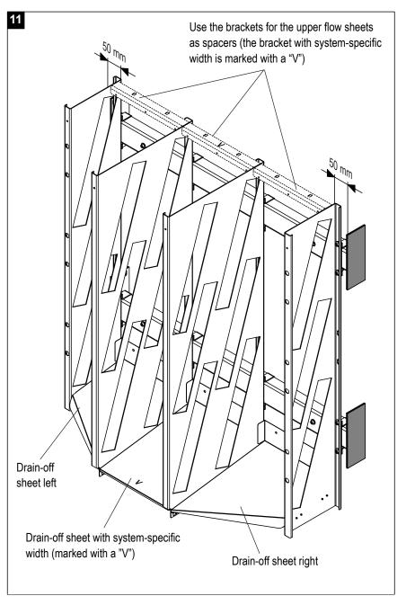
11. Use the clamping brackets to fix all vertical sections to the cross arms and temporarily align them according to the installation drawing provided.
