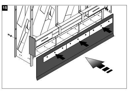
Cut the whole length of the tub sealing to the appropriate width (width = distance between upper edge of lower cross arm and bottom of duct plus 30 mm).
