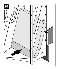
20. Insert in the lower flow sheet between the ceramic plate and the two vertical sections (this step must be carried out only for the lowest ceramic element of a vertical row).
