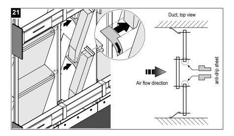
21. Only the rear rows of ceramic plates require the installation of anti-drip sheets. However, the anti-drip sheets must be installed only on the sides of the ceramic plates which overlap with the plates of a front row (see figure above). The ceramic plates at the very bottom require the installation of plate sealings instead of anti-drip sheets.
