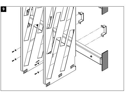
9. Fix the lower cross arm (lowest arm on systems with three cross arms) to the two vertical sections using the clamping brackets, the M6x20 hexagon socket screws and the washers supplied.
