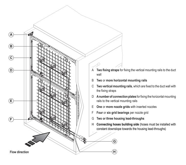
First fix the two vertical mounting rails on both sides in the duct (see installation drawing for positioning and fixing).
