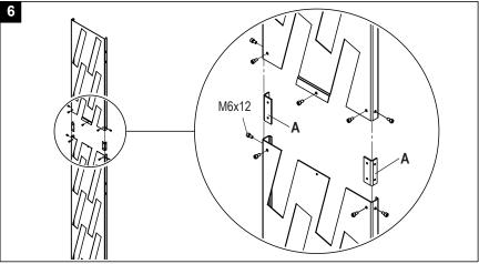
6. For systems with two-part vertical sections first connect all sections with the connector pieces "**A**" (2 pcs. per connection) and the M6x12 hexagon socket screws (9 pcs. per connection).
