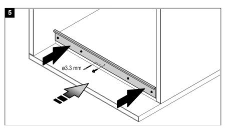
5. If your system is equipped with a "Booster", now mount the base plate in the tub. The base plate is attached to the tub ledge using self-tapping screws (drill holes ø3.3 mm before), behind the post evaporation unit.
