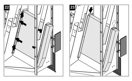
22. On each side insert the two-part lateral plate sealings. Proceed as follows: first insert the lower sealing piece between the vertical section and the ceramic plate, then push it downwards until it comes to a stop. Now insert the upper sealing piece and align its top end with the upper edge of the ceramic plate.
