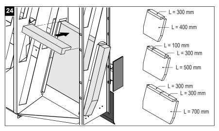
24. Place the ceramic angle (one or two angles) on top of the ceramic plate.
