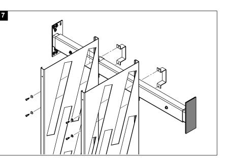
7. Fix each vertical section, left and right, to the upper cross arm, using the clamping brackets, the M6x20 hexagon socket screws and the washers supplied. The two vertical sections serve as spacers when mounting the lower cross arm.
