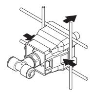
Squeeze the catch locks of the nozzle support and remove the support.
