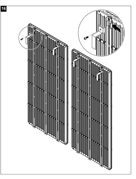
16. First fix the two upper brackets to all booster elements using the thread plates and the M6x12 mm hexagon socket screws (use topmost oblong holes).
