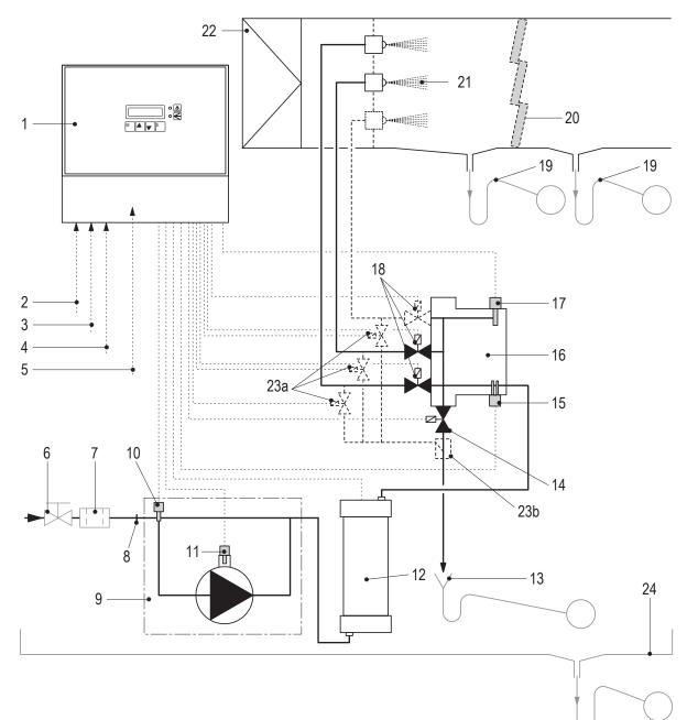
3.1 Basic design of the Condair Dual Hybrid Humidifier
