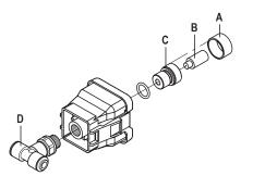
Loosen and remove nozzle (B) and nozzle adapter (C) by hand and the connection fitting (D) using an open-end wrench spanner (16 mm).
