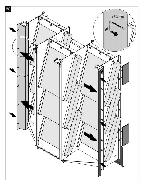
26. Fix the two-part lateral flow sheets to the duct wall using the self-tapping screws provided (drill holes Ø3.3 mm before). First mount the lower part of the lateral flow sheets, then the upper one (**the upper part must overlap the lower one**).
