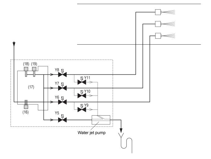
On systems having a central unit with spray circle discharge (option Z409) the spray circle drain valve Y5 opens after no humidification demand has occurred for 12 hours. Then, the valves Y9, Y10 and Y11 open one after the other for approximately 60 seconds to discharge each spray circle via the water jet pump.
