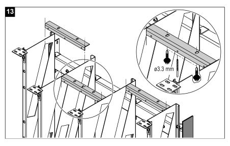
13. Mounting the brackets for the upper flow sheets:
