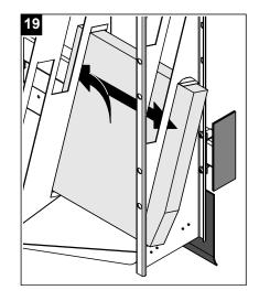
18. Insert the upper and lower plate sealings into the corresponding slots of the vertical sections and push them to the top or to the bottom respectively until they come to a stop (this fixes the plate sealings in position).
