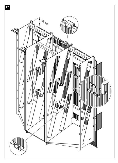
17. From the back, hang all booster elements to the upper cross arm. Use the thread plates and the M6x12 mm hexagon socket screws to fix the remaining brackets (2 or 4) to the booster elements (tighten the screws by hand only to allow later adjustment of the brackets).
