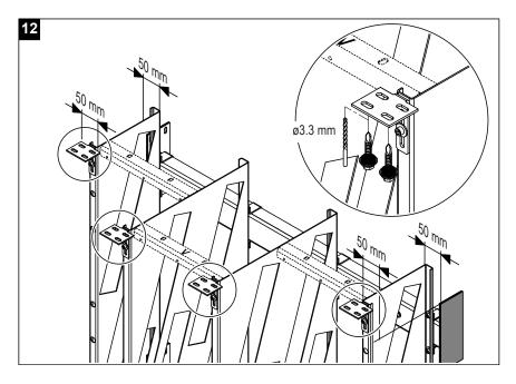
12. Mount the angle brackets to the upper end of all vertical sections and fix them with the M6x12 hexagon socket screws provided (slightly tighten by hand only).
