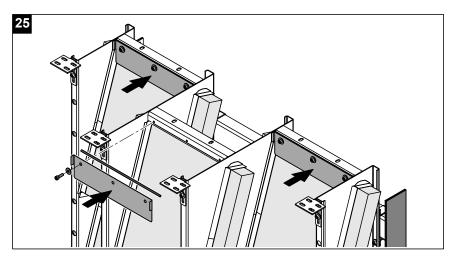
25. Cut the supplied rubber gasket band into pieces of the appropriate length. Use the supplied hexagon socket screws M6x12 mm and the washers to fix the upper flow sheets and the rubber gaskets to the brackets already installed.
