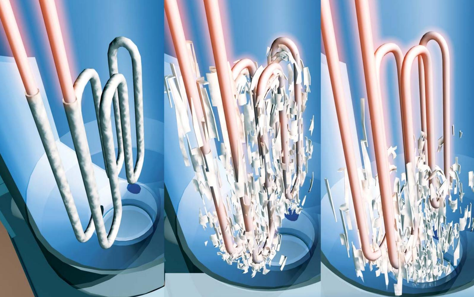
Scale is dislodged from the elements and falls into the scale collector tank
