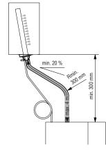
Initially, lead the steam hose with an **upslope of at least 20% over a minimum height of 300 mm**, then lead the hose with a **minimum upslope of 20%** and/or a **minimum downslope of 5%** to the steam distribution pipe.
