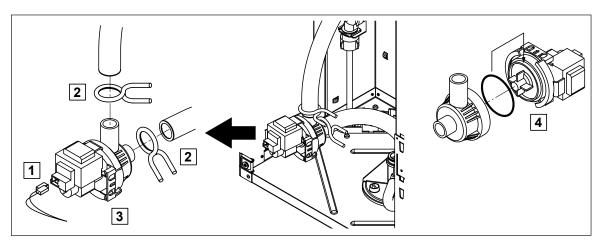
The steam cylinder does not need to be removed when removing the drain pump.
