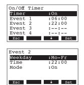
If the timer is activated, up to eight switching points (events 1 - 8) with different On/ Off events can be defined.
