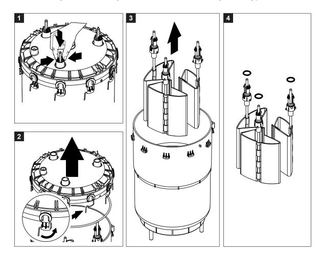
7.3.2 Disassembly and assembly of the cleanable steam cylinder type D...
