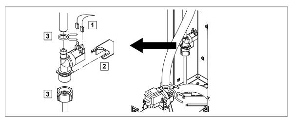
The steam cylinder does not need to be removed when removing the inlet valve.
