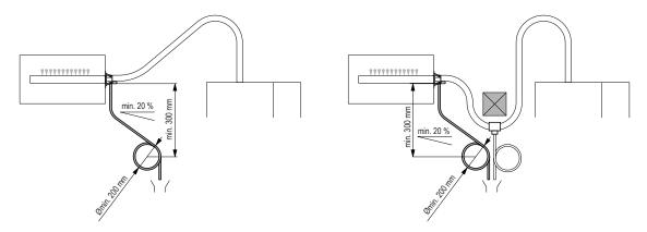
**Note**: If your unit feeds a number of steam distribution pipes, the individual condensate hoses are to be led into the discharge funnel.
